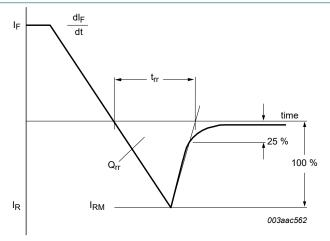
Fig. 12. Reverse recovery definition; ramp recovery
