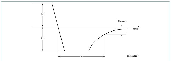
Fig. 11. Reverse recovery definition; step recovery
