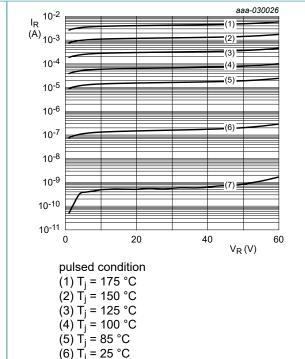
(7)  $T_j' = -40 \,^{\circ}\text{C}$ Fig. 4. Reverse current as a function of reverse
