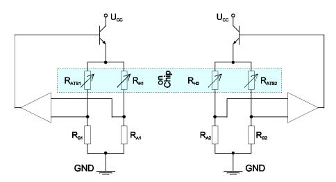
Above is shown an example of a measurement electronics using a Wheatstone-bridge.
