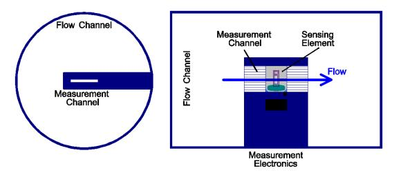
Flow channel of application example of a mass air flow sensor
