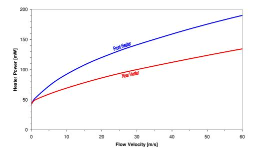
Example of a Power-Flow-Response of the LMM-H03
