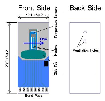
Mechanical dimensions and connections of LMM-H03
