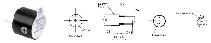
Dimensions : Millimetres Tolerance: ±0.5mm
