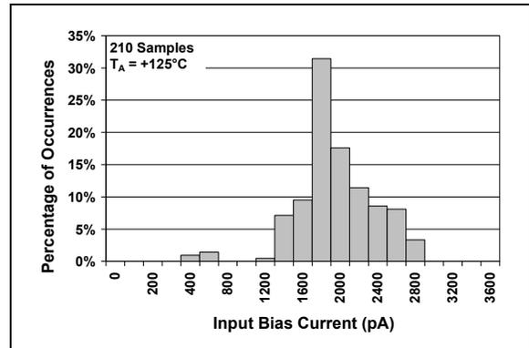
**FIGURE 2-5:** Input Bias Current at  $T_A = +125^\circ\text{C}$ .
