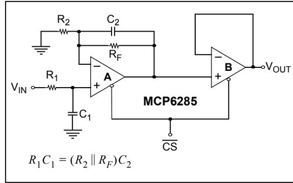
**FIGURE 4-13:** Buffered Non-inverting Integrator with Chip Select.
