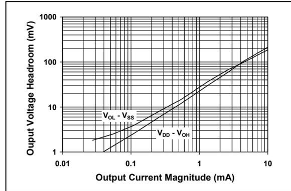
**FIGURE 2-16:** Output Voltage Headroom vs. Output Current Magnitude.
