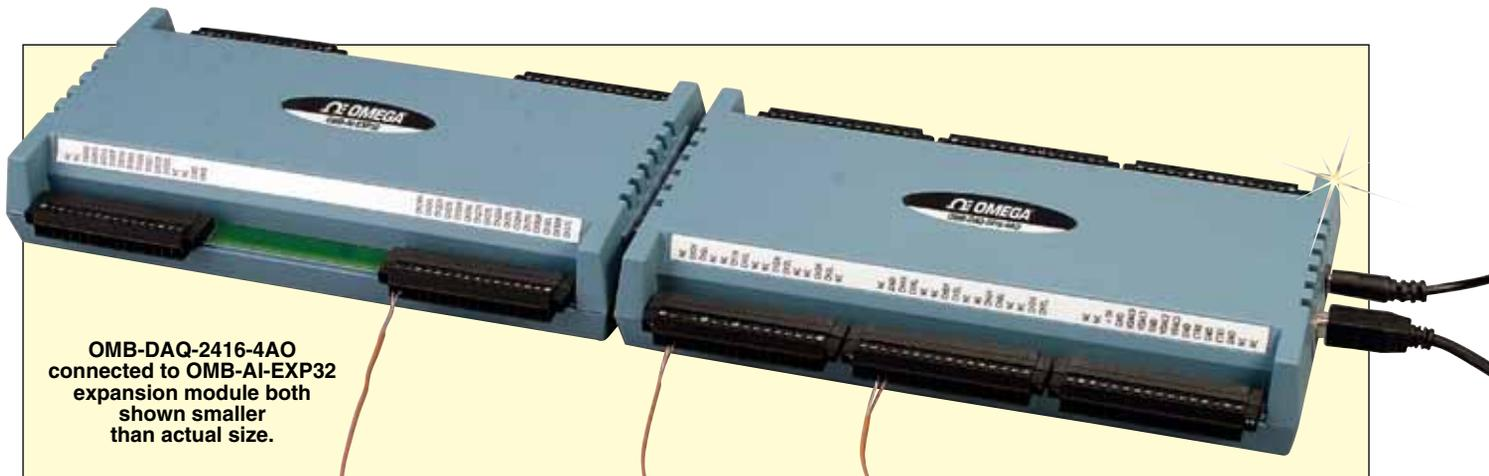
OMB-DAQ-2416-4AO connected to OMB-AI-EXP32 expansion module both shown smaller than actual size.
