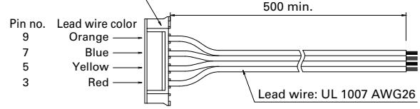
This motor cable is for model no. SF242□-10B□1.
