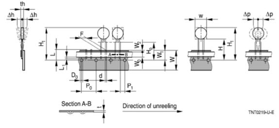
Dimensions and tolerances (taping in accordance with IEC 60286-2):
