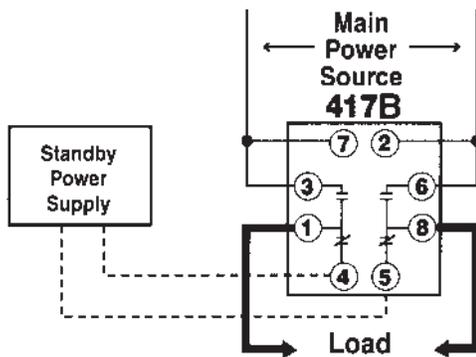
Controlled by a PLC, the 417B timing cycle can be aborted by using the remote reset terminals.
