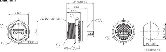
Panel Cut-Out Dimensions: Millimetres
