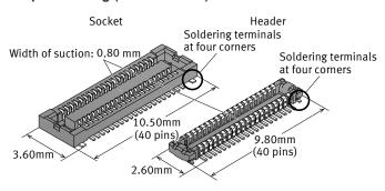
■ High resistance to various environments! "TOUGH CONTACT" construction provides high contact reliability
