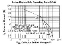
There are two limitations on the power handling ability of a transistor average junction temperature and second breakdown safe operating area curves indicate  $I_{\rm C}$  - V<sub>CE</sub> limits of the transistor that must be observed for reliable operation i.e, the transistor must not be subjected to greater dissipation than the curves indicate
