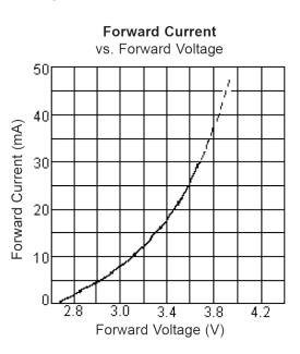
White Typical Electrical Optical Characteristics Curves (T<sub>A</sub> = 25°C Ambient Temperature Unless Otherwise Noted)
