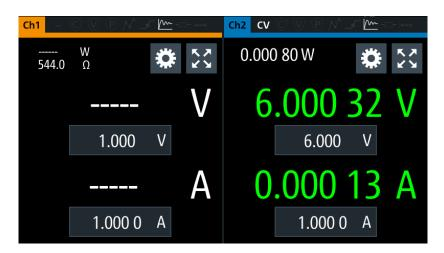
Figure 6-3: Output of Ch2 in CV mode
