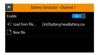
Figure 6-12: Battery simulator dialog
