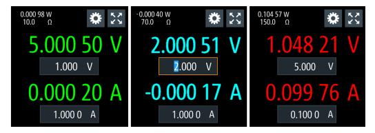
Figure 5-3: Color coding of operating conditions
