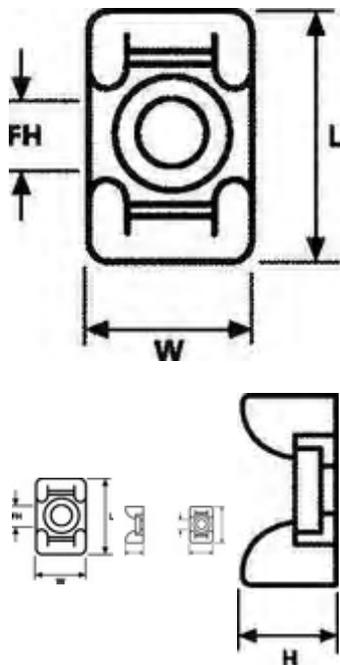
KR mounts give additional support to the cables by means of their curved design. Simple to install with a screw or bolt they give excellent security, particularly in areas of high vibration when used in conjunction with the KR straps. They must offer one of the most vibration resistant fixings available.
