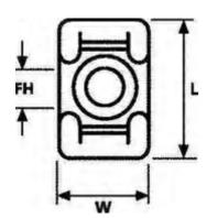
Both CT & KR mounts give additional support to the cables by means of their curved design. Simple to install with a screw or bolt they give excellent security, particularly in areas of high vibration - when used in conjunction with the KR straps (see page ??) must offer one of the most vibration resistant fixings available.
