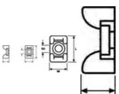
Designed specifically for holding heavier cable bundles these mounting bases can be used in many industries from agriculture to truck manufacture, they offer a very secure fixing and can be used with a wide variety of heavy duty cable ties up to 7.6mm wide.
