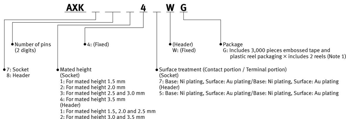
Note: 1. Only a socket of mated height 3.5 mm: 2,000 pieces embossed tape and plastic reel packaging × 2 reels
