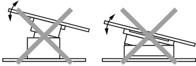
■ Keep the PC board warp no more than 0.03 mm in relation to the overall length of the connector.
