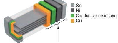
Termination consists of 4 layers including conductive resin layer.
