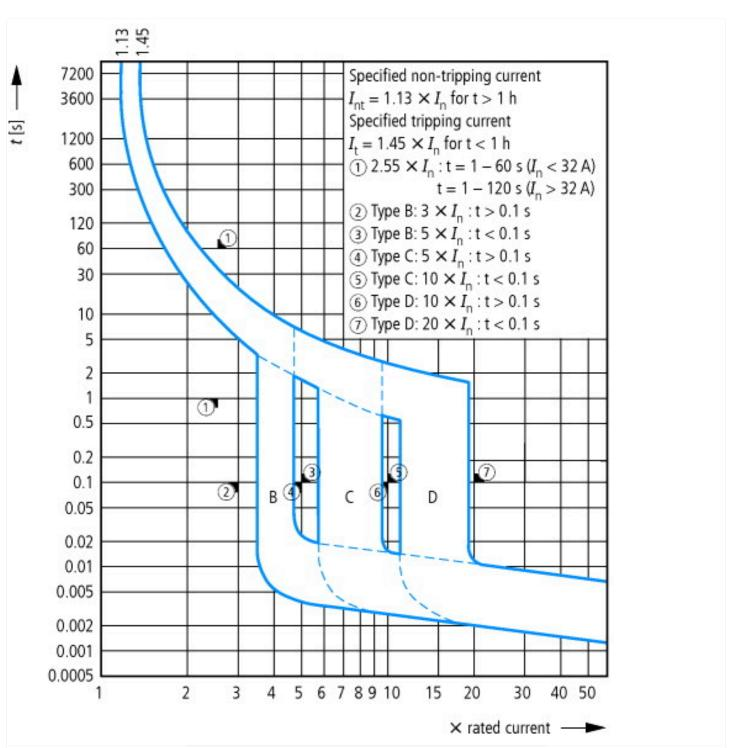
Tripping characteristic at 30 °C: B, C, D to IEC/EN 60898
