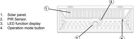
Press the button one or more times to set the mode of operation. The corresponding indicator LED lights. When there is no operation of more than 30 seconds setting mode is cancelled and the indicator LED extinguishes.
