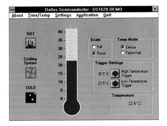
The DS1620K demonstration kit allows a potential user of the DS1620 to observe the operation of the DS1620 in an actual temperature measurement application. Temperature is measured and displayed in a text box, as well as on a graphical thermometer. Thermostat trippoints may be set by the user, and a graphical display of the status of each thermostat output is available on the screen at all times. Temperature may be displayed in Celsius or Fahrenheit.
