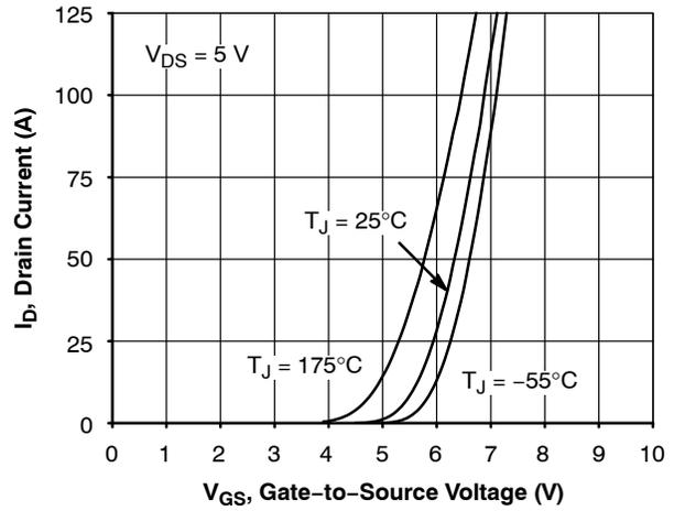
Figure 2. Transfer Characteristics
