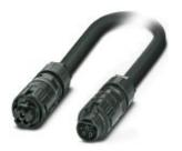
Circular connectors (cable-side), Range of articles: PRC, Connecting cable, housing material: PPE, color: black, number of positions: 3, nom. voltage: 690 V AC, rated current: 24 A, Connection method: Screw connection, Type of contact: Socket/pin
