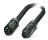
Circular connectors (cable-side), Range of articles: PRC, Connecting cable, housing material: PPE, color: black, number of positions: 5, nom. voltage: 690 V AC, rated current: 32 A, Connection method: Screw connection, Type of contact: Socket/pin
