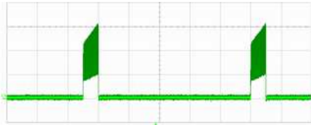
Locked rotor current @ 24 V ( I = 0,2\text{A/div} ; t = 1\text{s/div} )
