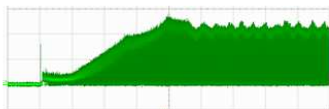
Start-up current @ 24 V ( I = 0,5\text{A/div} ; t = 2\text{s/div} )
