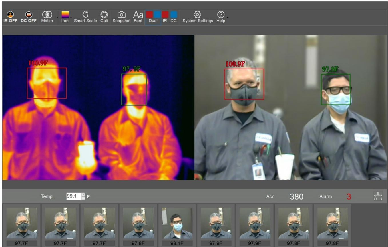
Also the software gives visual and sound alarms when a high body temperature is detected. The high body temperature individual will have a red square appear around their face and a sound will be triggered.
