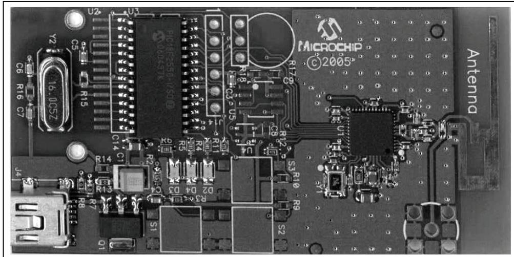
The ZENA Wireless Network Analyzer uses a USB mini-B cable to connect to the PC. The ZENA analyzer is powered by the USB bus. A PCB trace antenna receives the packets on the specified channel and sends the information over USB to the PC computer using the HID standard class.
