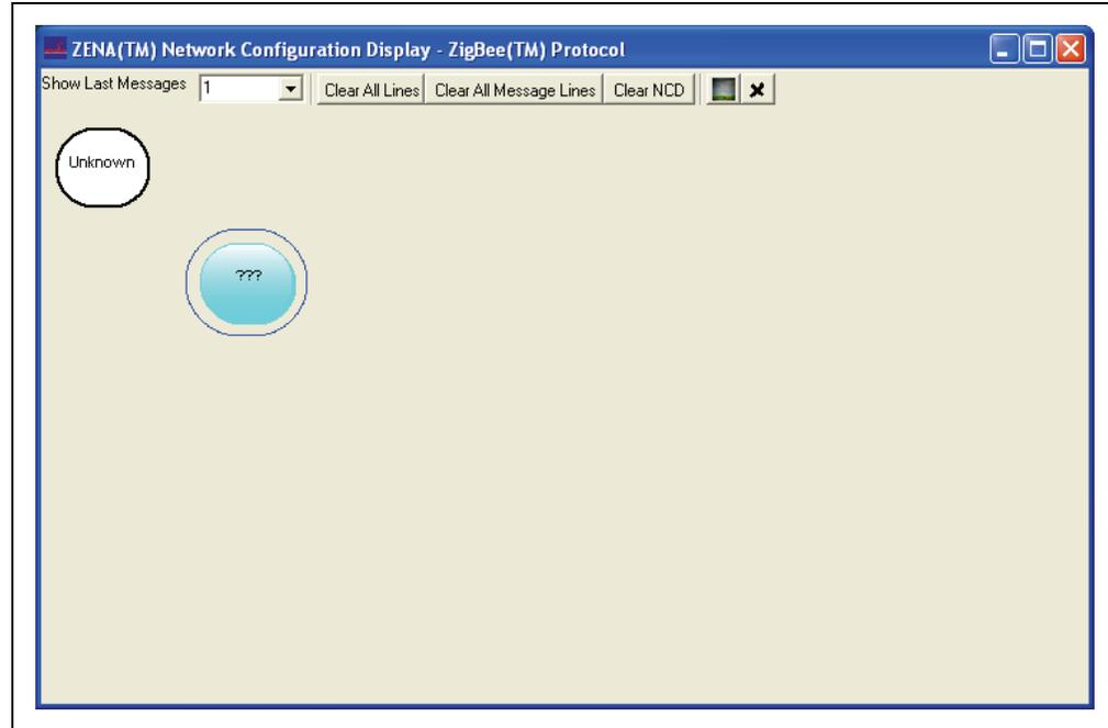
Note that the ZENA analyzer can tell from the beacon that this device is a ZigBee protocol coordinator, but it does not yet know its MAC address.
