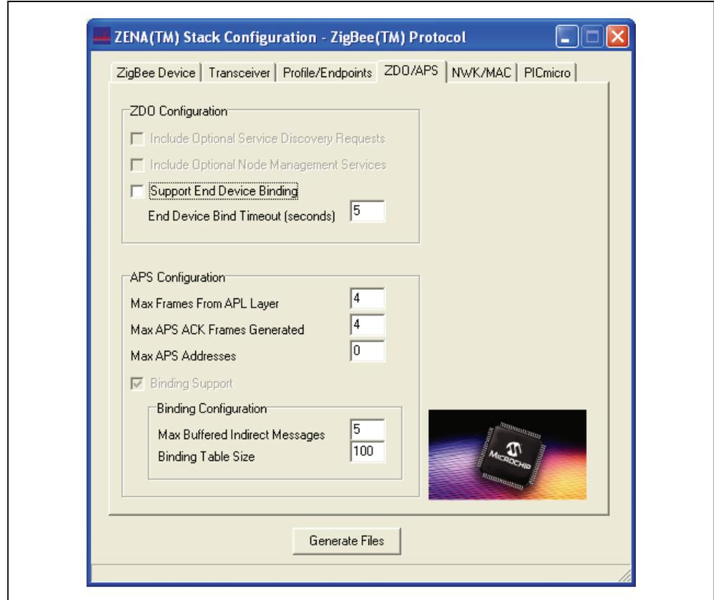
This tab is used to configure the ZDO (ZigBee Device Object) and APS (Application Sub-Support) stack layers. Many options on this tab are enabled or disabled based on the “ZigBee Device Type” specified on the **ZigBee Device** tab.
