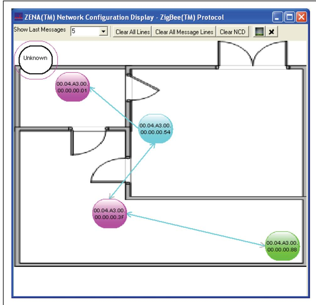
**FIGURE 3-28: APS ACKNOWLEDGE PATH WITH FLOOR PLAN BACKGROUND**
