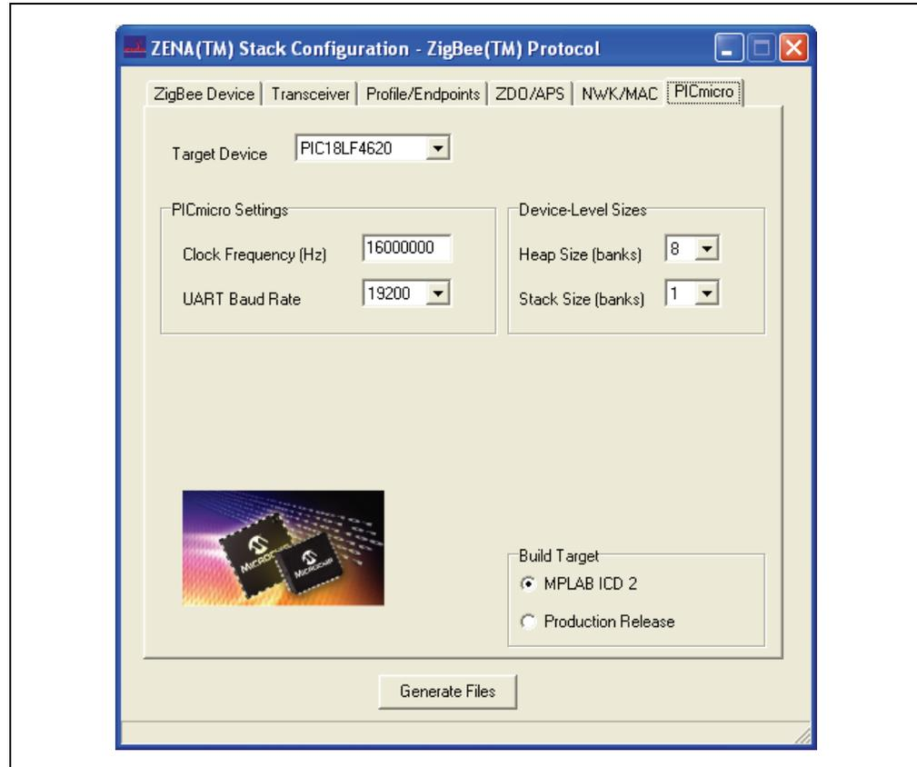
This tab is used to configure basic PICmicro MCU options (see Table 3-8).
