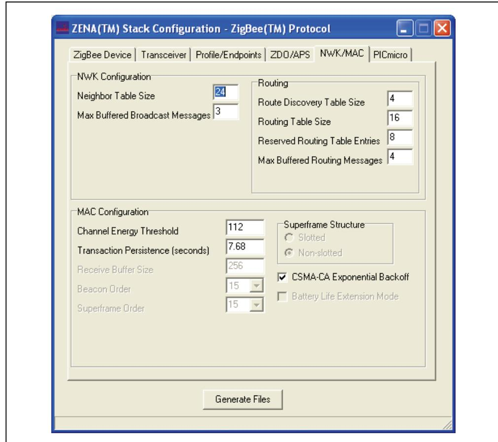
This tab is used to configure the NWK (Network) and MAC (Medium Access Controller) Stack layers. Many options on this tab are enabled or disabled based on the “ZigBee Device Type” specified on the **ZigBee Device** tab.
