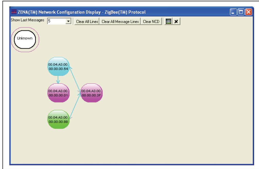
The NCD window shows how the message went from device 00.04.A3.00.00.00.88 to device 00.04.A3.00.00.00.01, traveling through two other nodes.
