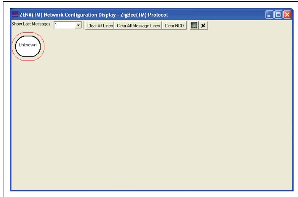
Since there are no nodes on this channel, no beacons are received, and the ZigBee protocol coordinator forms a network.
