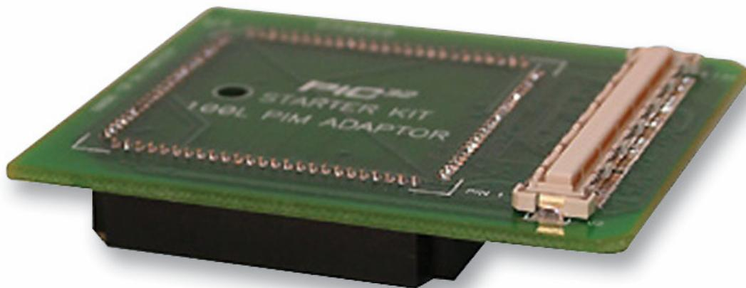
This adapter enables PIC32 Starter Boards to connect to the Plug-In Module on Explorer 16. Users can utilize the functionality on the Explorer 16 or connect PICTail Plus daughter cards for application-specific development.
