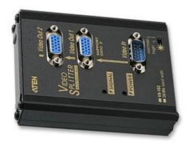
These devices are the simplest solution for SVGA and VGA signal distribution. By cascading them an infinite number of monitors displaying the same image can be achieved. These standard resolution splitters cater for monitors with bandwidths up to 250 Mhz. The distribution units incorporate signal boosters which enhance the video signal for long distance broadcasting; up to 35m.
