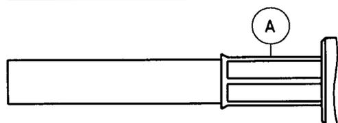
Slide ferrule A over braid and crimp as close to connector body B as possible.
