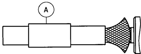
Splay out braid and insert cable in connector body B.
