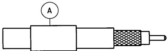
Taper cable centre contact to a point with the tip trimmer W 264.
