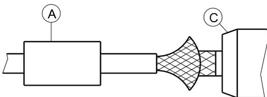
Splay out braid and insert cable in connector body C. Ensure that braid lies above the crimp neck.
