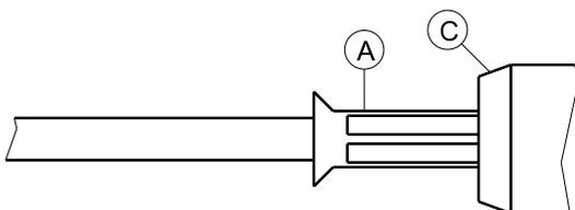
Slide ferrule A over braid and crimp as close to connector body C as possible.
