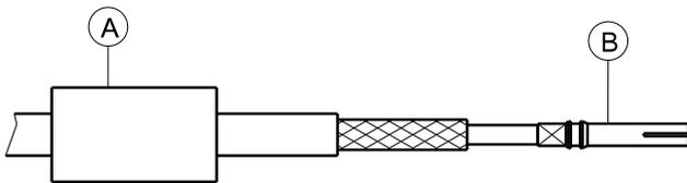
Push contact B over inner conductor of cable to abut dielectric and crimp.
