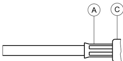
Slide ferrule A over braid and crimp as close to connector body C as possible.
