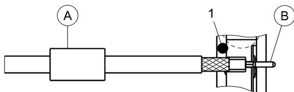
Push contact B over inner conductor of cable to abut cable dielectric and crimp with insert 1.
