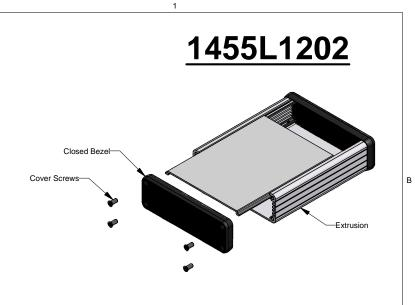
Note Purchased assembly includes box, belly plate, bezel, cover screws and self dhesive rubber feet. Box made from Extruded Aluminum 6063. PART NUMBERS L1202 Clo Clear Anodize 1455L1202 Black Anodized 1455I 1202B ACCESSO Cover Screws (Pkg 100) [#6 Self Tapping Nickel Plated Screws] Black Cover Screws (Pkg 100) 1455MS100 1455MS100BK [#6 Self Tappng Nickel Plated Screws Bezels, Biack (Pkg 10) HAMMOND MANUFACTURING ,, 1455LPLBK-10 Closed Plastic www.hammondmfg.com
