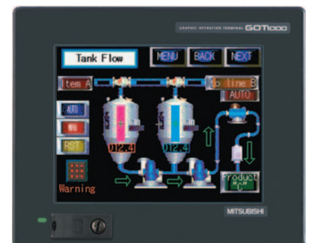
The GOT is a typical HMI
