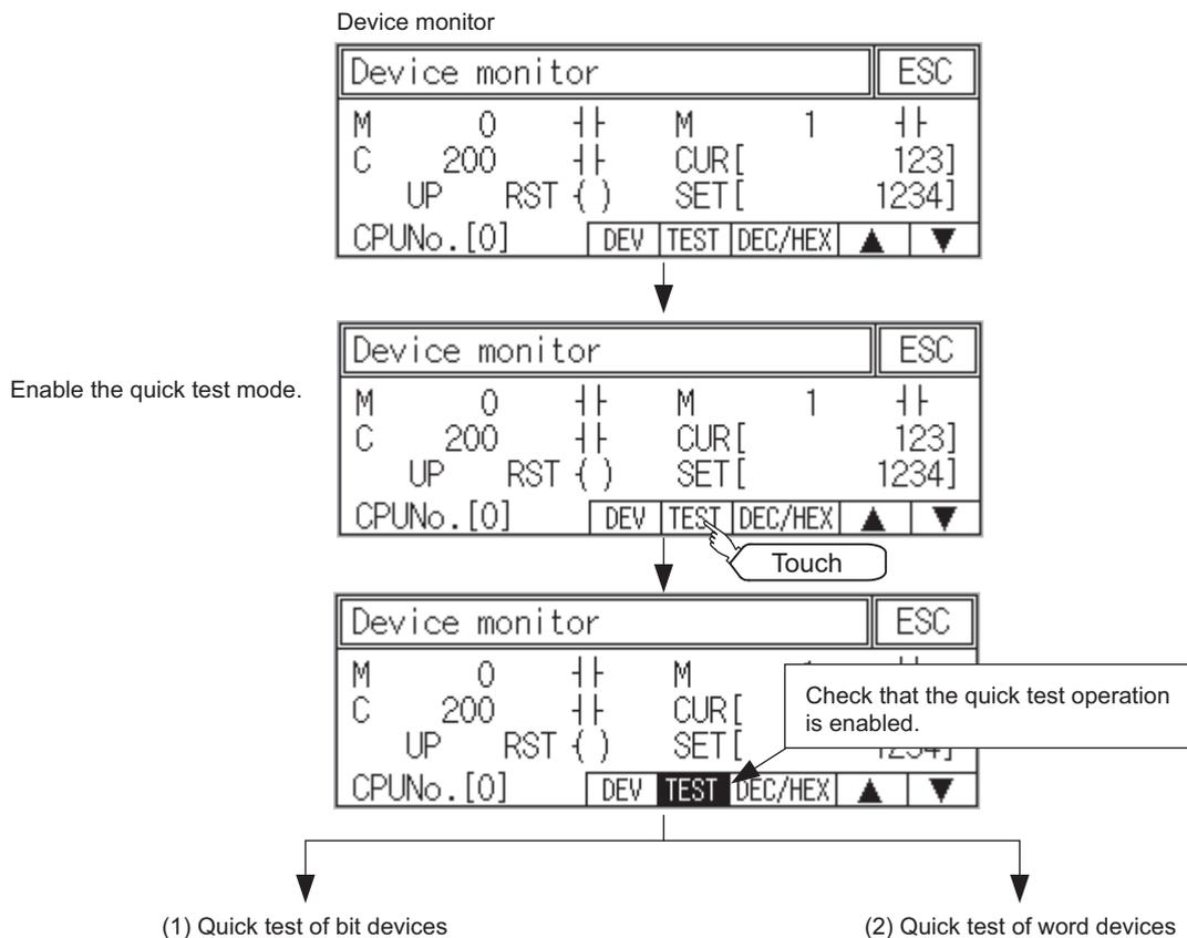
(1) Quick test of bit devices
