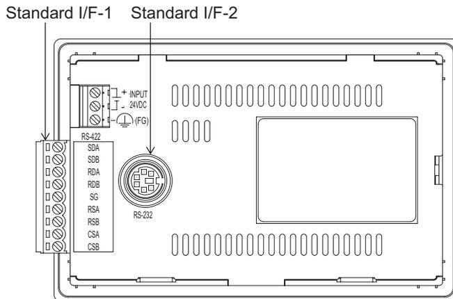
Whether an RS-422 or an RS-232 interface (Standard I/F-1) for communication with PLC is used depends on the GOT model.
