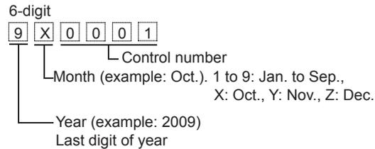
The production date of the optional replacement battery can be confirmed by the lot No. marked on the nameplate (label) affixed on the battery.
