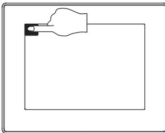
1 Power OFF the GOT, and attach the memory board which stores the standard OS and communication driver to the GOT.
