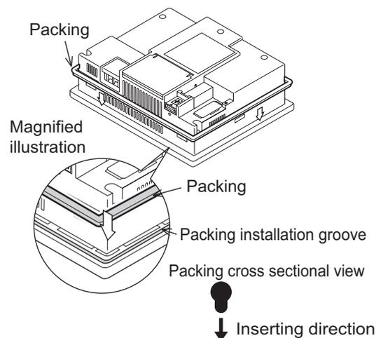
**2** Inserting into the panel face
