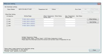
**4.** Mark the checkbox of the channel where offset and gain values are to be set, and click [Offset Setting] button.
