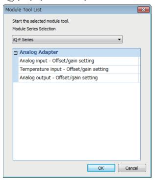
**1.** In "Analog Adapter", select "Analog input - Offset/gain setting" and click [OK] button.
