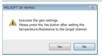
**7.** Apply the gain temperature to the terminal of the corresponding channel, and click [Yes] button.
