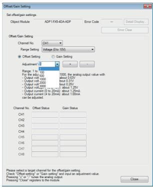
**6.** The adjustment value of the offset value or gain value can be selected from "1", "100", "500", "1000", "2000", and "3000" or it can be set by inputting any value (1 to 3000).
