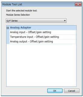
In "Analog Adapter", select "Temperature input - Offset/ gain setting" and click [OK] button.
