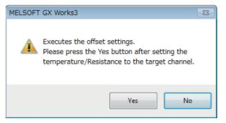
**5.** Apply the offset temperature to the terminal of the corresponding channel, and click [Yes] button.
