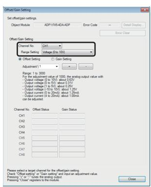
**4.** Specify the channel to configure the offset/gain setting and the user range setting.
