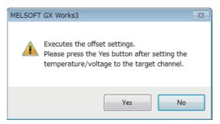
**5.** Apply the offset temperature to the terminal of the corresponding channel, and click [Yes] button.
