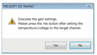
**7.** Apply the gain temperature to the terminal of the corresponding channel, and click [Yes] button.
