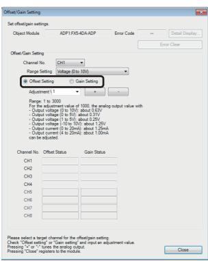
**5.** Use the radio button to specify whether to perform the offset setting or gain setting. (Step 6 and later describe the case when the offset setting is specified.)
