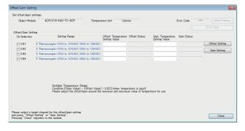
**4.** Mark the checkbox of the channel where offset and gain values are to be set, and click [Offset Setting] button.
