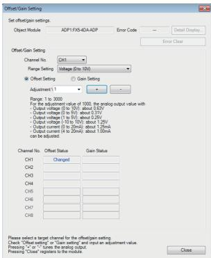
output voltage or analog output current value corresponding the set adjustment value.
