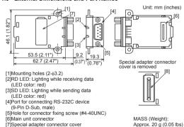
The communication port of the FX3U-232-BD is a 9-Pin D-Sub male type. The table below shows the pin arrangement.
