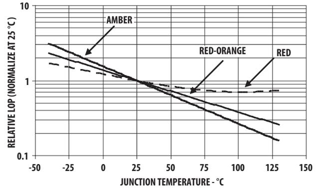
Figure 9. Relative Light Output vs Junction temperature
