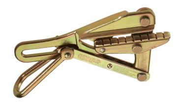
Klein Tools' 1611 Series Chicago Grips have a round inside jaw contour designed to hold weatherproof strand and solid coated wire. They also have a notched jaw to provide a firm grip on insulation. All Klein grips are manufactured from custom drop-forged steel that is machined and heat treated for excellent durability. Each grip is individually hand inspected and actuated for proper function. Grips are also rigorously tested and pulled to rated load to ensure the highest quality and reliability.
