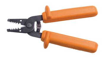
This compact, lightweight wire-stripping, cutting tool cuts, strips, loops and gauges solid wire. Dual layer orange-over-white insulation protects against electric shock. Meets or exceeds ASTM F1505-10, IEC 60900: 2004, CAN/ULC-60900-09, NFPA 70E, 2011 ed., CSA Z462 standards for insulated tools, and are clearly marked with the official 1000-volt rating symbol. Hardened spring steel with precision-ground stripping holes for easy removal of insulation.
