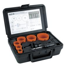
The Bi-Metal Hole Saw Kit contains the most popular sizes for basic electrical work plus two arbors. Multiple leverage points provide easy slug removal. Heavy duty bits bore through 2x4s in a single pass. All in a rugged carrying case.
