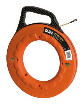
Designed for flexibility and easy navigation through conduit runs, this spiral steel fish tape slides easily over existing wires and through multiple bends. The durable spiral steel tape construction yields a maximum pulling force of up to 500-pounds (227 kg). The polypropylene case and handle are extremely durable and offer the maximum in shock and impact resistance.
