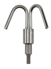
The Twin Hook Attachment is a replacement part for both the 7-Piece Fish Rod Attachment Set (Cat. No. 56511) and the 33-Foot Fish and Glow Rod Kit (Cat. No. 56400). This durable stainless steel grappling-style hook works well on its own or threaded on the end of the Whisk Attachment (Cat. No. 56513) in areas crowded with other wires or cables. This attachment fits all Klein fish and glow rods. Note: Does not fit Super Rod Series (SRS) fish rods.
