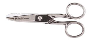
These Electrician Scissors are nickel plated with wire stripping notches for 19 and 23 gauge wire. Blades hardened to 58C Rockwell for extra cutting life with serrations for holding wire while it cuts. High-quality blades produce a sharp, clean, uniform cut.
