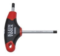
The Klein JTH6E13BE 1/4-Inch Hex Ball-End Journeyman T-Handle features a T-Handle design that delivers more torque to the fasteners. The part number and hex size appear on the handle for easy, positive identification. Molded-in finger grooves provide a more comfortable grip.
