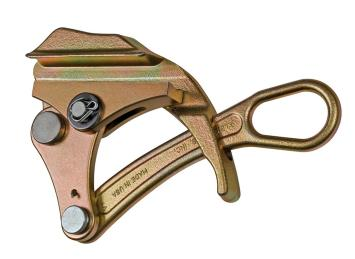
Lightweight, compact grips pull an exceptionally wide range of cable sizes and types. Designed with a round serrated jaw to firmly grip insulated cables and conductors. A hot latch closed automatically to guard against grip accidently disengaging from wire. A large opening in the handle accommodates a wide variety of hooks on hoists, winches and tackle blocks.
