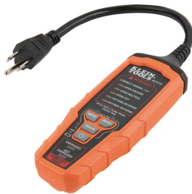
RT310 is an electrical tester that tests the wiring condition at an electrical outlet, and inspects and checks AFCI and GFCI devices. It is designed for use with North American 120V electrical outlets. It can detect and identify common wiring faults. Includes 3 x 1.5V AAA alkaline batteries.
