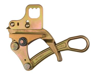
The Klein KT4802 Forged Parallel Jaw Grips with Hot-Latch's large round eyelet opening in the handle is perfect for accommodating a wide variety of hooks on hoists, winches and tackle blocks. The hot latch closes automatically to guard against grip accidently disengaging from the wire. The KT4802 has a jaw length of 5-1/8 - Inches.
