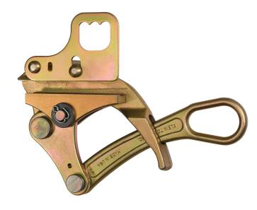
The Klein KT4502 Forged Parallel Jaw Grips with Hot-Latch's large round eyelet opening in the handle is perfect for accommodating a wide variety of hooks on hoists, winches and tackle blocks. The hot latch closes automatically to guard against grip accidently disengaging from the wire. The KT4502 has a jaw length of 3-Inches.
