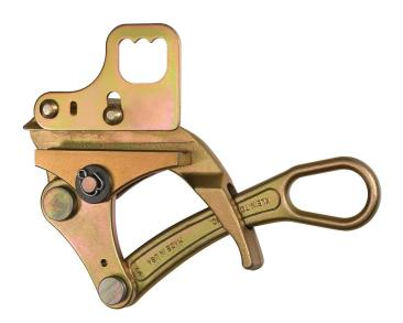
The Klein KT4602 Forged Parallel Jaw Grips with Hot-Latch's large round eyelet opening in the handle is perfect for accommodating a wide variety of hooks on hoists, winches and tackle blocks. The hot latch closes automatically to guard against grip accidently disengaging from the wire. The KT4602 has a jaw length of 5-Inches.
